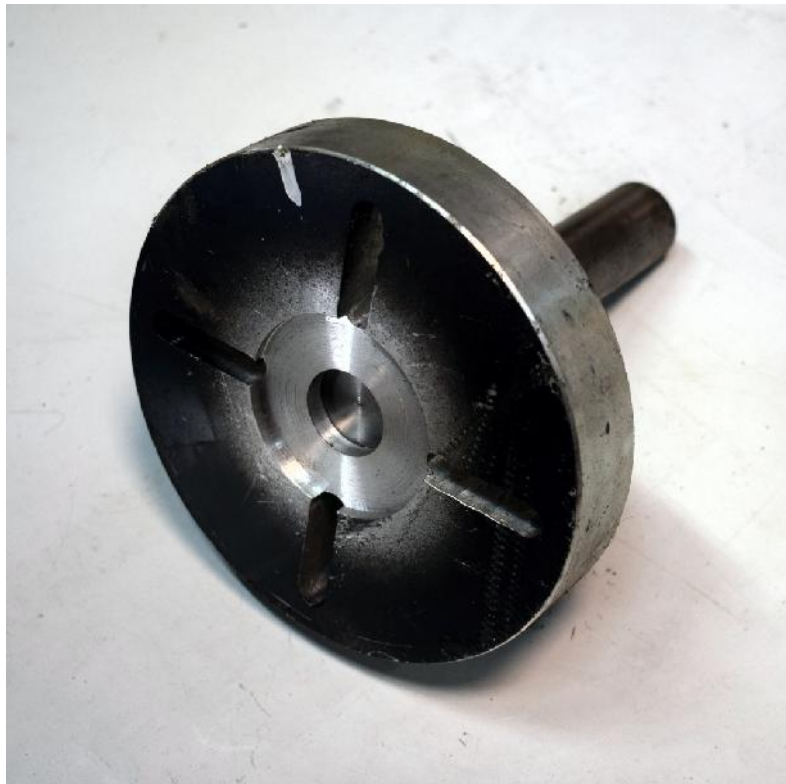
Driveline adapter for flange yoke
