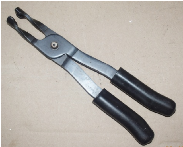
Heavy Duty Seal Gripper Pliers Serrated tangs for secure grip Like new Goodson or K-line (i forget)
