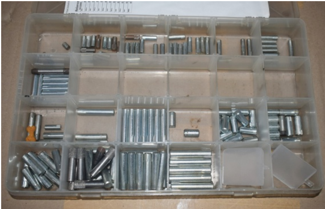
Balance pins for Harmonic Balancers, flywheels & Clutch Covers
