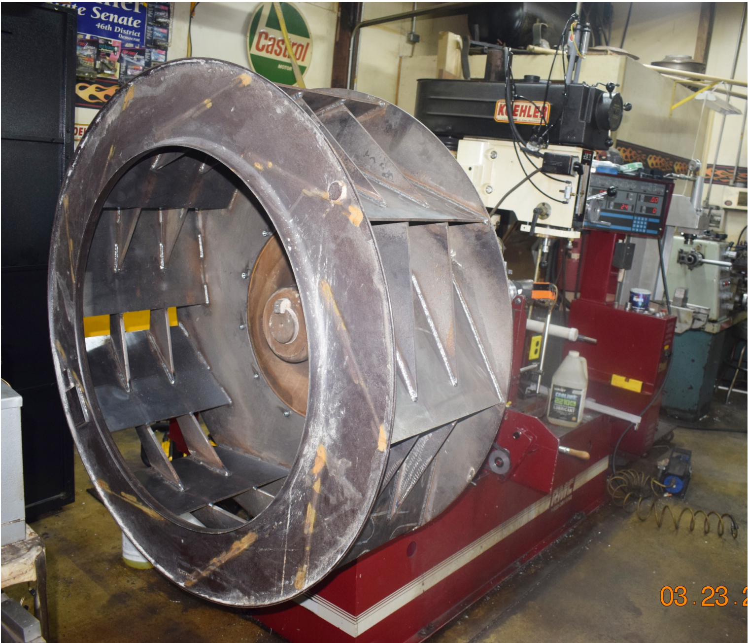
Extra large hand fabricated impeller
