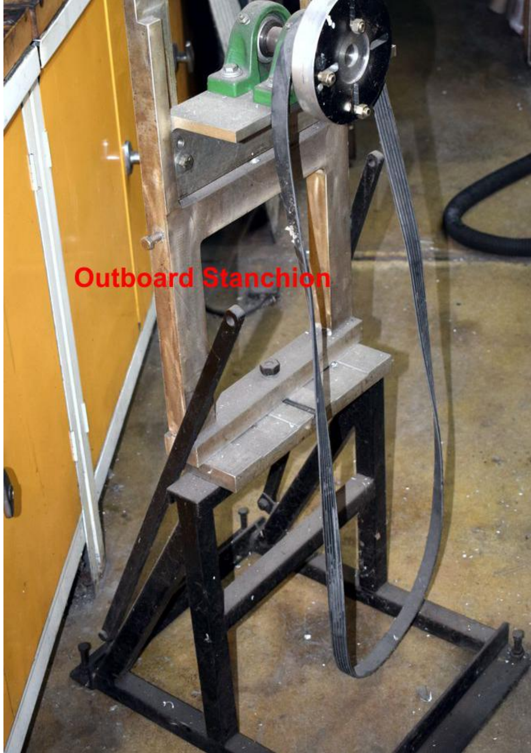
Outboard Stantion For things longer than the bed. Shown with driveshaft flange end adapter.
