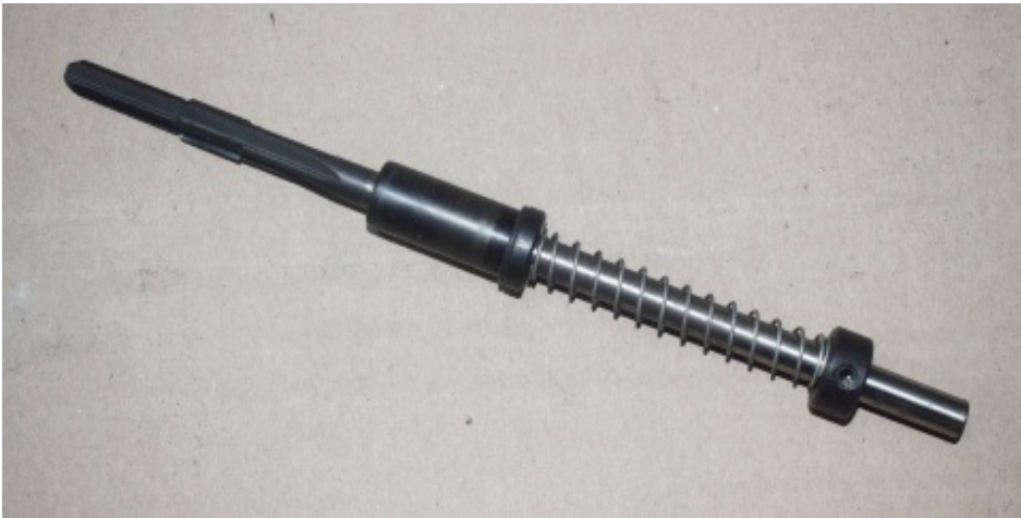
KL8570 3/8 boring for use with seat centering cones
