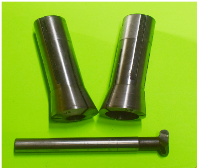
R8 Collets 1/2 & 3/4" Special cutter for piston metal removal.
